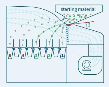
The ASM aerodynamic separator separates any material of a certain density with a high accuracy of +/- 3%.
